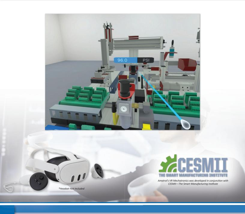
Amatrol's VR Smart Factory - Allen-Bradley (VR870-AB) creates a digital twin of Amatrol's three-cart Mechatronics training system that can be explored virtually via a Meta Quest VR headset. Users can observe the operation of the system that assembles a working industrial directional control valve, including pneumatic pick and place feeding, go/no-go gauging/quality inspection (height and orientation verification), and automated inventory/parts storage.
