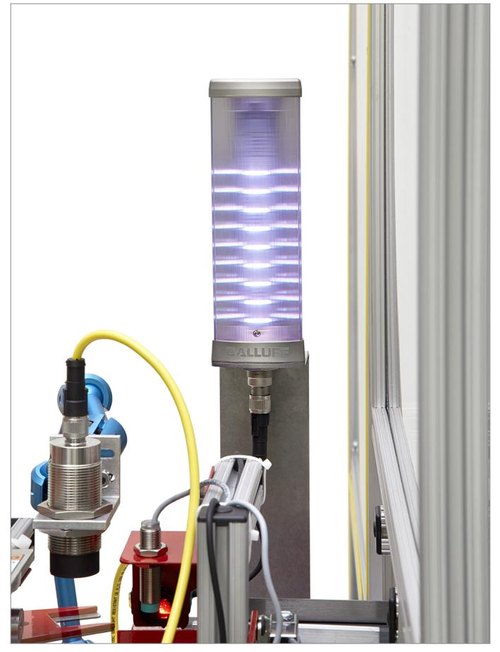
This system teaches PROFINET (Siemens) network communications between a stack light and other smart automation devices in a Smart Factory environment to efficiently control and monitor automated manufacturing processes.
